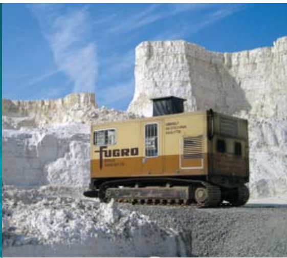
Cone Penetration Testing, Germany. Geophysical applications of CPT include UXO mapping and investigation of ground anchors and sheet pile depth using magneto cone sensors.
