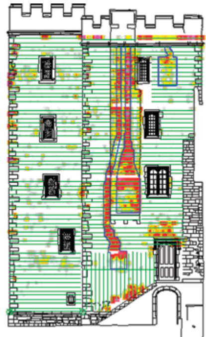
Mapping voids in masonry walls, UK
