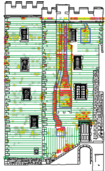
Mapping voids in masonry walls, UK
