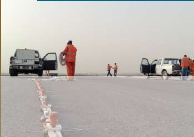
MASW survey, Abu Dhabi
