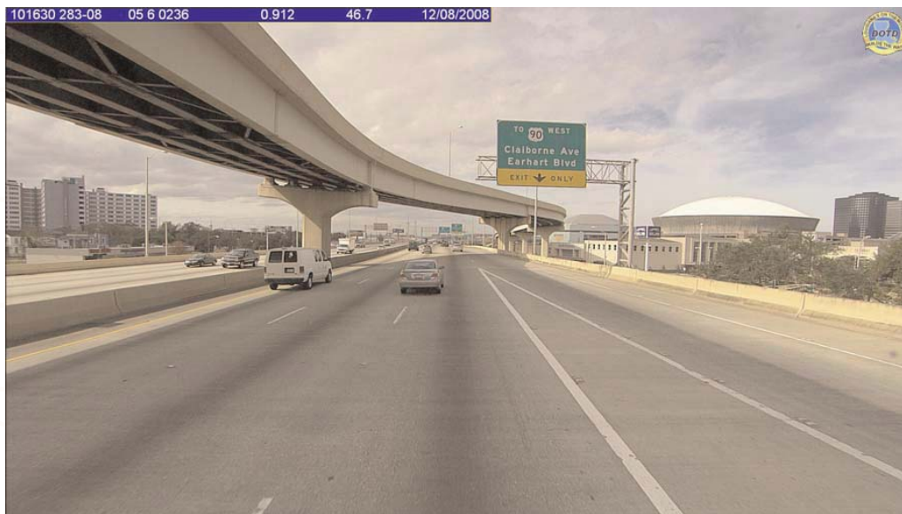
Pictured here: 1920 x 1080 pixel resolution (HD) Right-of-Way video image, with 90 degree horizontal field of view
