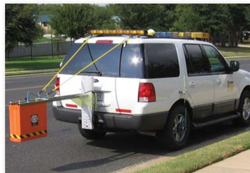
Ground Penetrating Radar (GPR)
