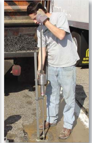
Dynamic Cone Penetrometer (DCP)
